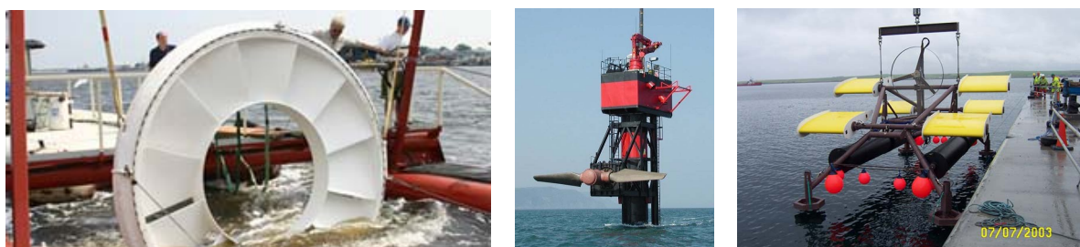
Figure 1: Prototype testing of tidal current energy devices: (i) OpenHydro Group Ltd., (ii) MCT's Seaflow, (iii) RGU's SeaSnail
