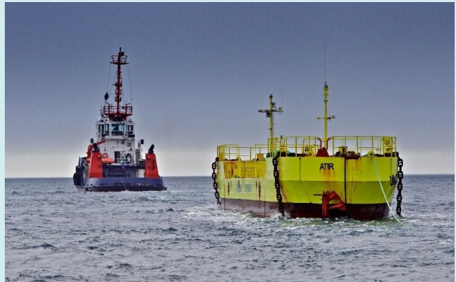
Installation of Magallanes ATIR tidal platform at EMEC's Fall of Warness tidal test site (Source: Colin Keldie)
