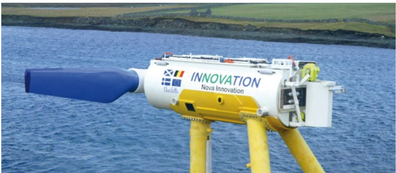
Nova M100 turbine, installed in the Shetland Tidal Array (Photo credit: Nova Innovation)
