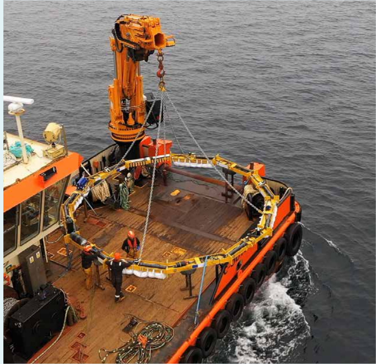
RealTide Advanced Turbulence Sensor (Source: University of Edinburgh & EMEC)
